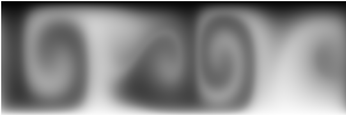
Figure 4.5: Destabilising the uniform temperature gradient
